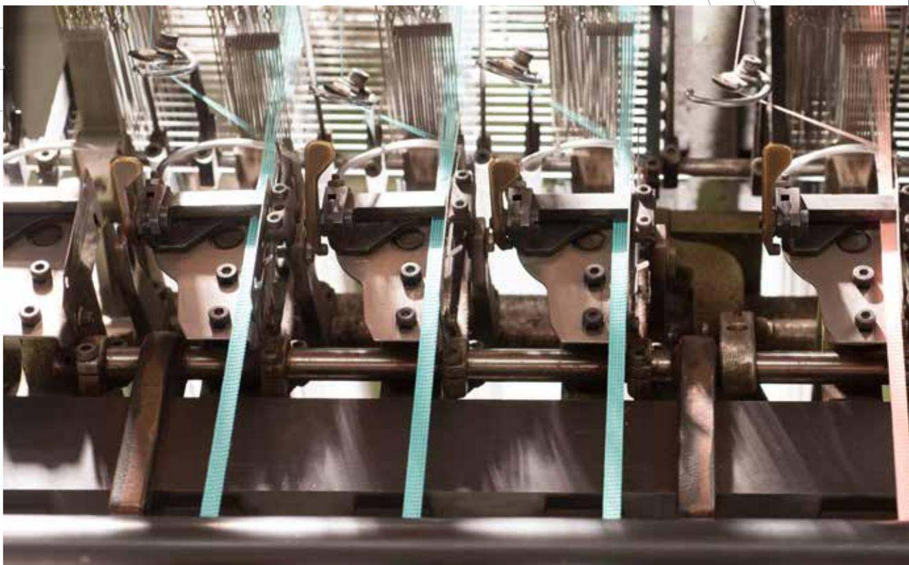
Drive belt and change gear to perform stabilized transmission of bottom weft and provide wider range of fabrics which be more superior in quality.
