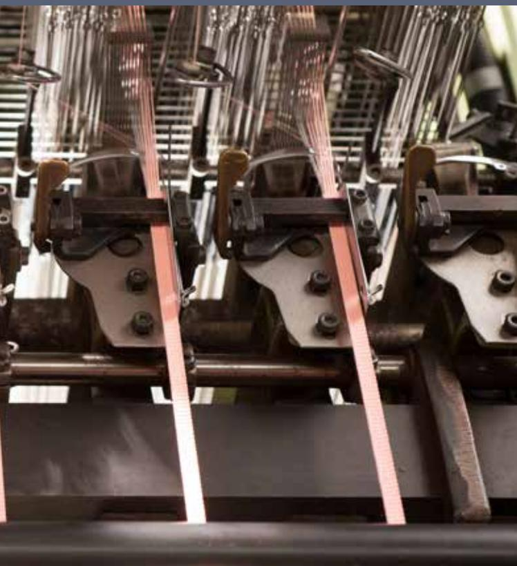
Convertible machine parts supported with various devices to provide wider range of fabrics multi-purpose for single machine as well. Heald frame in double-load, double-shedding lever, twin pattern chain transmission configuration of shaft and gear has been reinforced.
