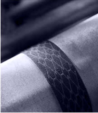
With Jacquard webbing machine, we can create patterned effect using computerized control system. Commonly used in sandals and bag accessories, this automated patterned technique can also be used on elastic webbing, usually used in undergarment.
