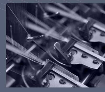
Drive belt and change gear to perform stabilized transmission of bottom weft and provide wider range of fabrics which be more superior in quality.
