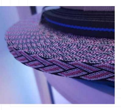
Jacquard looms can be programmed, making the weaving process much more versatile and allowing for a higher degree of control of the warp yarn. It makes it possible to automatically produce unlimited varieties of weaving patterns, including webbing. The process can also be used for Jacquard webbing, patterned knitwear and machine-knitted textiles.
